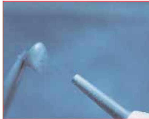
Removing the oxide by sandblasting
